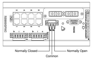
Figure 2.7. Failsafe Output Relay
